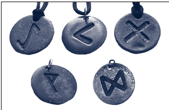
FIGURE. Medallions from recalled toy necklaces that were sold in vending machines in Oregon and linked to lead poisoning
