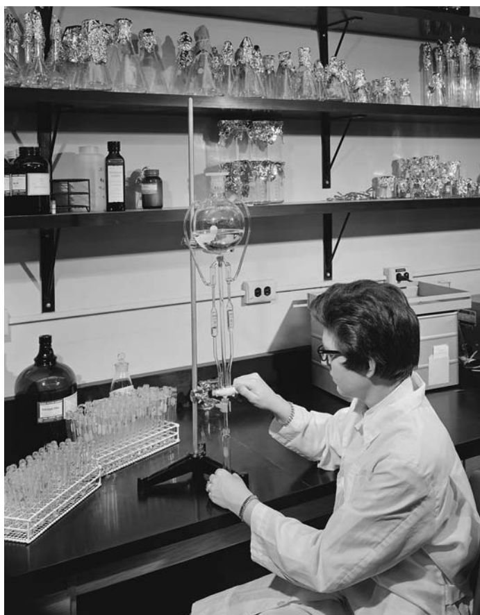
FIGURE 3. A laboratorian using a manual method for conducting a cholesterol determination. 1966
